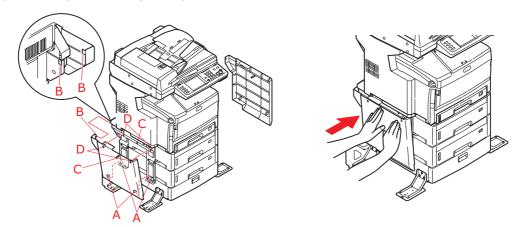
**8.** Clip stabilizing foot covers into position ensuring you align locating lugs and grooves as shown.
